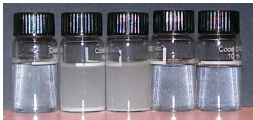
Figure 10: Photo of five of the Phosphate test vials. Note that the darker the blue hue, the greater the phosphate levels
