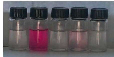
Figure 7: Photo of five of the Chlorine test vials. Note that the darker the pink hue, the greater the chlorine level
